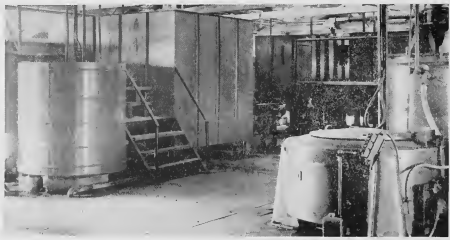
Part of the factory layout is shown in the above picture. The tanks at the left are the chemical separation units; the tanks at the rear receive the juice when it is first mixed with sea water, and the machine in the foreground in the high-speed centrifuge dryer.
